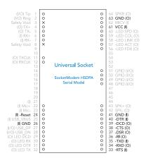
Universal Socket Connectivity. Multi-Tech's universal socket is a flexible, comm-port architecture that provides cellular, Ethernet, PSTN or Wi-Fi network access with interchangeable communications devices. This means you can utilize one system design and populate it with your connectivity device of choice accommodating multiple connectivity requirements. In addition, you are assured a seamless migration to future technologies.
