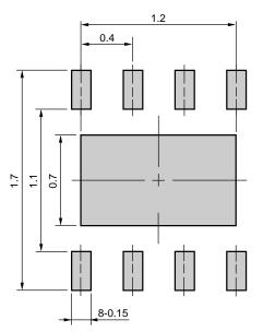
Remark The mounting pad layout in this document is for reference only. When designing PCB, please consider workability of mounting, solder joint reliability, prevention of solder bridge and so on, in order to optimize the design.
