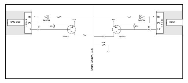
Figure 1. Typical Circuit for Single-line Serial Communication Bus
