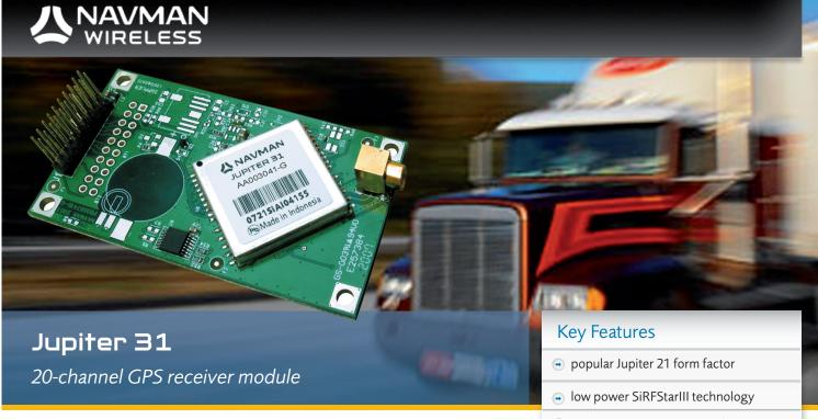
The Jupiter 31 is a 20 channel GPS receiver module based on the Jupiter 21 form factor that is significantly enhanced to take advantage of the SiRFStar III architecture. The Jupiter 31 offers a substantial increase in sensitivity, faster time to fix, lower power consumption and the option of using either an active or passive antenna.
