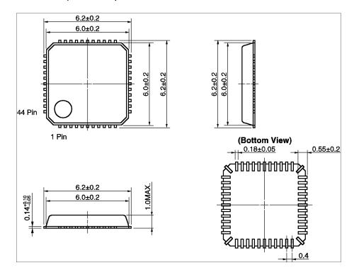
Caution The island pins located on the corners are needed to fabricate products in our plant, but do not serve any other function. Consequently the island pins should not be soldered and should remain non-connection pins.
