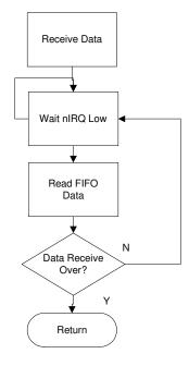
After Initialisation, open FIFO receive mode and wait for nIRQ low, only then can the MCU read received and stored data in FIFO. For the next received package please reset FIFO
