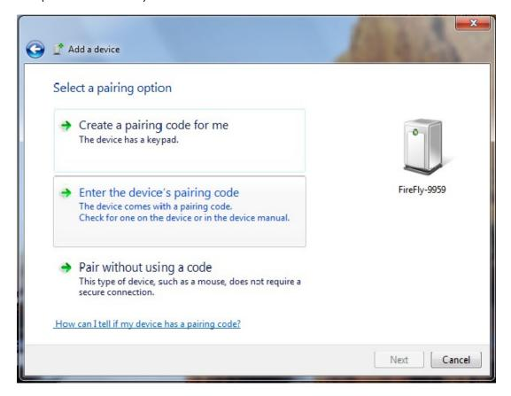
**Connecting:** To establish a Bluetooth connection, open up the COM port assigned to the device from either your application or a terminal emulator. Once the COM port is open you will notice the green LED switches from blinking to solid ON. The device will remain connected until the COM port is closed or the FireFly BP is turned off.
