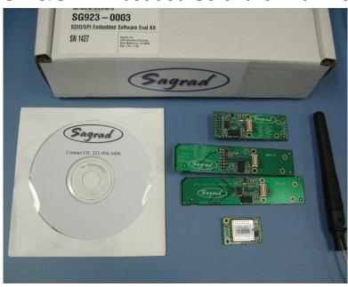
The SG923-0003 SDIO/SPI Embedded Software Eval Kit is a software integration evaluation kit for the SAGRAD Wi-Fi SG901-1039 fully integrated 802.11b & g ultra-low power Wi-Fi radio module. The evaluation kit includes all the hardware necessary for successful software integration. Processor and O/S specific drivers may be available from SAGRAD. It is recommended that the user contact SAGRAD directly for information regarding available Processor and O/S specific drivers.
