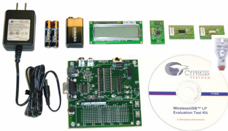
FIGURE 2. WirelessUSB LP EVK contents including platform board, MiniProg, modules, batteries, and adapter
