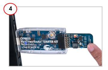
Connect the PC dongle to your PC and slide down the CapSense slider to check the output. The tricolor LED lights up in different colors depending on the finger position
