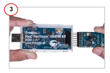
Connect the multifunction card to the PC dongle.
