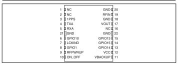
Figure 2: SG Series Receiver Pinout (Top View)
