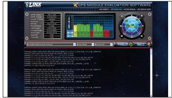
Figure 7: The SG Series Master Development System Software
