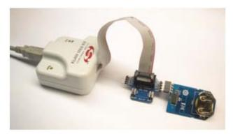
In this setup, the user can incorporate the debugging capabilities into the final application using a cheap 4-pin header connection. Silicon Labs' ToolStick USB Debug Adapter (not part of the development kit) is also compatible with the key fob development platform and can be used in the above scenarios.
