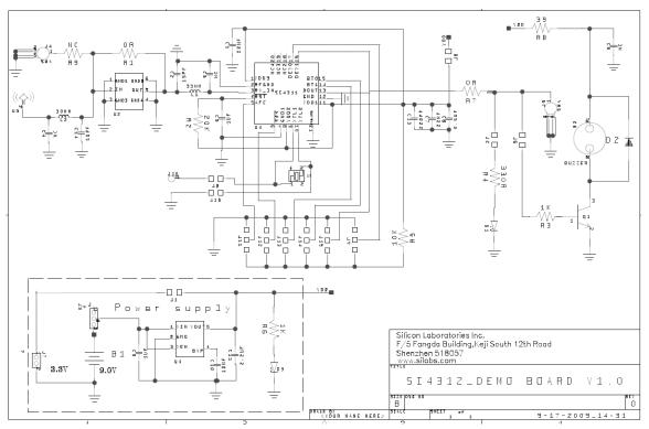
Figure 3. Si4312-DEMO Schematic
