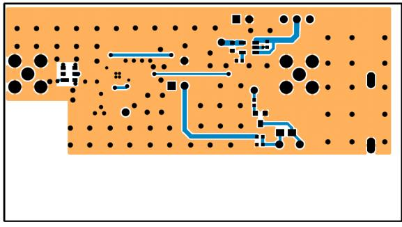
Figure 5. Si4312 PCB Bottom Layer
