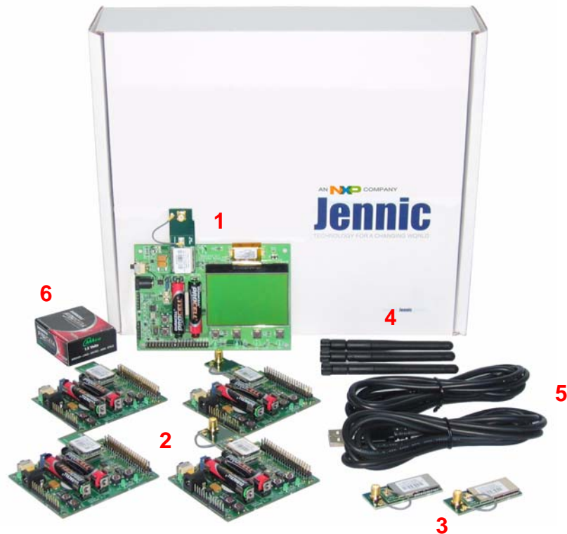
Figure 1: JN5148-EK010 Evaluation Kit Components
