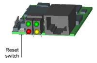
**Note:** The reset switch is in same location for both wired and wireless modules.
