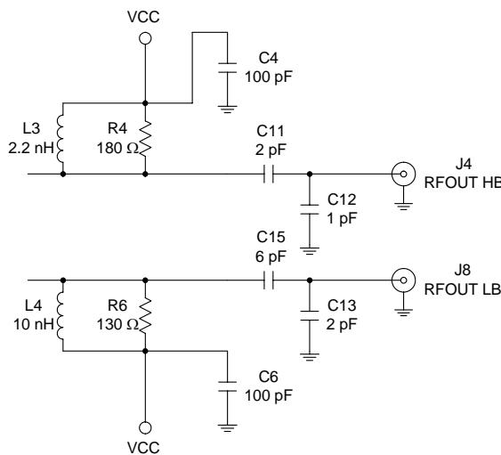
Figure 1. Alternate RF output match with third-harmonic suppression.
