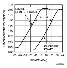
FIGURE 3. Typical power detector response, V<sub>OUT</sub> vs. PA output Power
