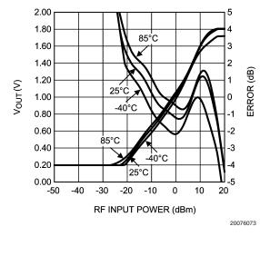
Output Voltage vs. RF Input Power (LMV228 in LLP) 2.50 900 MHz 2.25 1800<sup>'</sup>MHz 2.00 1900<sup>'</sup>MHz 1.75 1.50 S V<sub>out</sub> ' 1.25 1.00 2000<sup>'</sup> MHz 0.75 0.50 0.25 0.00 -50 -40 -30 -20 -10 0 10 20 RF INPUT POWER (dBm) 20076070 Output Voltage and Log Conformance vs. RF Input Power @ 1800 MHz (LMV228 in LLP) 2.00 1.80 85°C 1.60 3 1.40 2 ERROR (dB) 1.20 Vout (V) 25<sup>°</sup> 1.00 n -40°C 0.80 0.60 -2 85°C 0.40 -3 -40°C 0.20 .4 25 °C
