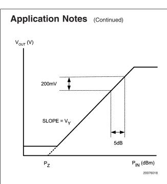
FIGURE 5. VOUT vs. RF Input Power PIN
