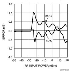
Output Variation vs. RF Input Power Normalized to 25°C @ 1900 MHz (LMV228 in microSMD)
