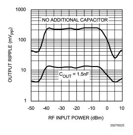
FIGURE 6. Output Ripple vs. RF Input Power
