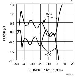
**Output Variation vs. RF Input Power** Normalized to 25°C @ 2000 MHz (LMV225)
