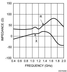
RF Input Impedance vs. Frequency @ Resistance and Reactance (LMV225 in micro SMD)
