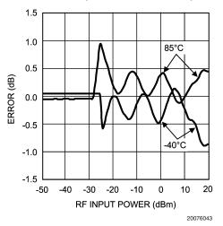
Output Variation vs. RF Input Power Normalized to 25°C @ 2000 MHz (LMV228 in microSMD)
