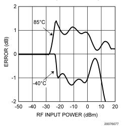
Output Variation vs. RF Input Power Normalized to 25°C @ 2000 MHz (LMV228 in LLP)
