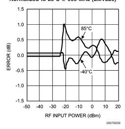
**Output Variation vs. RF Input Power** Normalized to 25°C @ 1900 MHz (LMV226)
