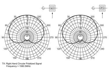
**NOTE 1:** Center frequency is shifted approximately 5MHz down when covered with a radome.
