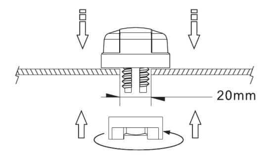
Recommended torque for mounting is 95Nm or 70ftlbs Maximum torque for mounting is 135.6Nm or 100ft lbs
