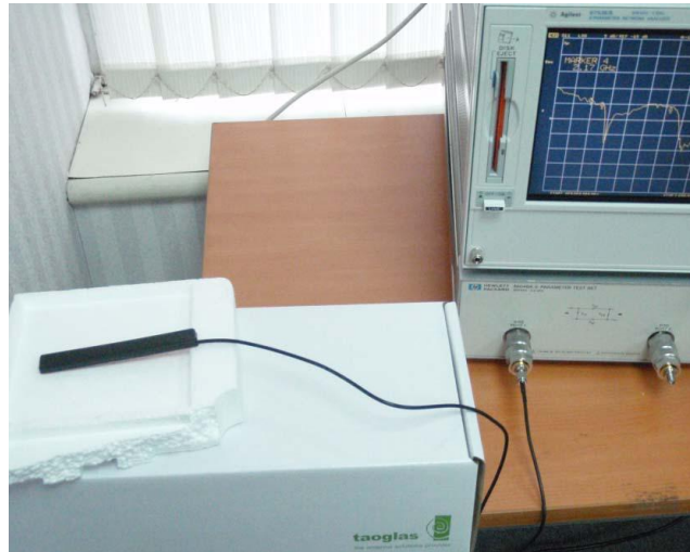
Free space Return Loss measurement setup
