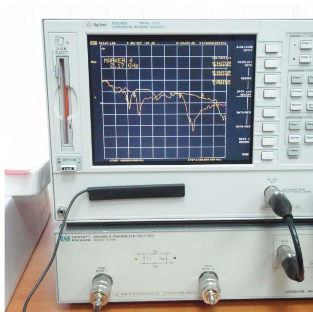
Free space Return Loss measurement setup
