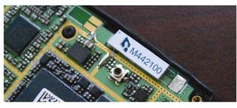
These highly innovative antennas provide competitive advantages for designers of cell phones, laptops and other mobile equipment by combining GPS & Bluetooth antennas in a single, highly compact form factor suitable for the thinnest/smallest devices. Ethertronics Isolated Magnetic Dipole (IMD) technology utilizes superior RF isolation to combine these two high performance antennas.
