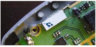
Ethertronics' Savvi series of Isolated Magnetic Dipole<sup>™</sup> (IMD) antennas deliver on the key needs of device designers for higher functionality and performance in smaller/thinner designs. These innovative antennas provide compelling advantages for GPS enabled cell phones, navigation equipment, and other mobile devices.
