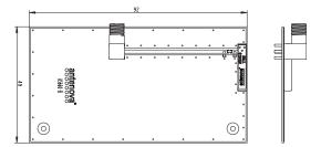
The testboard is designed for evaluation purposes for Mica 2.4 GHz SMD antenna. The board has the same size as a typical PCMCIA card and is fitted with an SMA connector.
