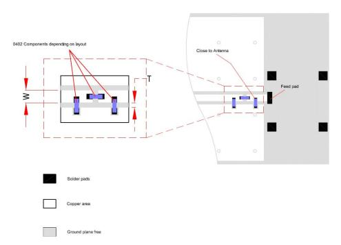
The antenna feed pad and the antenna ground pad are indicated in the drawing above. Additional pads are for mechanical attachment only and should not be grounded.
