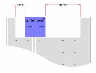
Additional ground and components near the antenna should be at a distance of at least 5 mm from the left hand side and 18 mm or more from the right hand side as shown in the drawing above.
