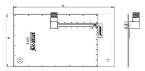
The testboard is designed for evaluation purposes for Rufa 2.4 GHz SMD antenna. The card has the same size as a typical PCMCIA card and is fitted with an SMA connector.
