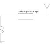
The testboard is matched with above specified component.
