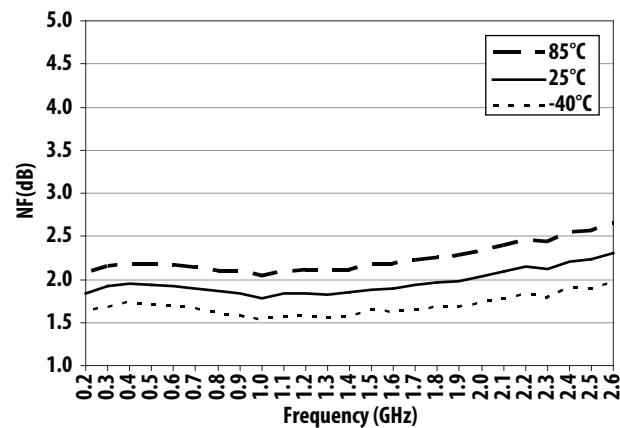
Figure 21. Noise Figure over Frequency and Temperature
