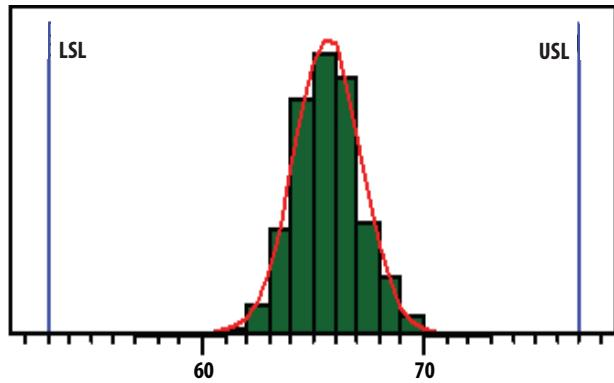
Figure 1. I<sub>ds</sub>, LSL=53mA , nominal=65mA, USL=77mA
