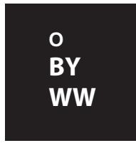
Note: Package marking provides Orientation and identification:
