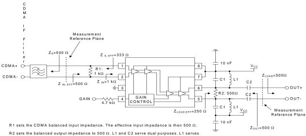
R2 sets the balanced output impedance to  $500~\Omega$ . L1 and C2 serve dual purposes. L1 serves as an output bias choke, and C2 serves as a series DC block. In addition, the values of L1 and C2 may be chosen to form an impedance matching network of the load impedance is not  $500~\Omega$ . Otherwise, the values of L1 and C1 are chosen to form a parallel-resonant tank circuit at the IF when the load impedance is  $500~\Omega$ .
