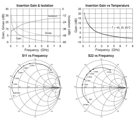
Note: S-parameters are de-embedded to the device leads with  $Z_s = Z_L = 50\Omega$ . The data represents typical performace of the device. De-embedded s-parameters can be downloaded from our website
