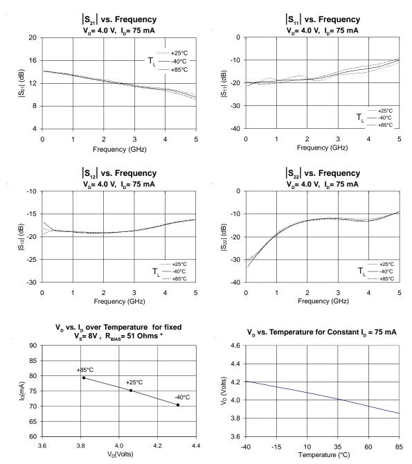
\* Note: In the applications circuit on page 4, R<sub>BIAS</sub> compensates for voltage and current variation over temperature.
