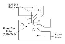
Use multiple plated-thru via holes located close to the package pins to ensure a good RF ground connection to a continuous groundplane on the backside of the board.
