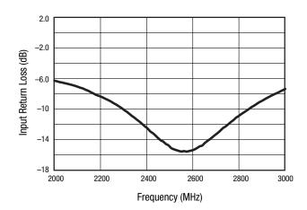
Figure 4. Input Return Loss vs Frequency Over Temperature (PiN = -20 dBm)
