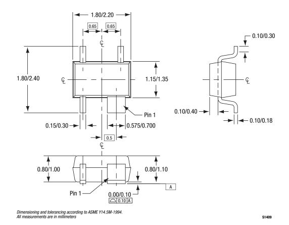
Figure 12. SKY65052-372LF 4-Pin SC-70 Package Dimensions
