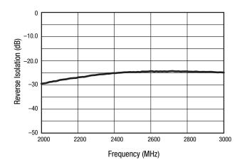
Figure 5. Reverse Isolation vs Frequency Over Temperature ( $P_{IN} = -20 \text{ dBm}$ )
