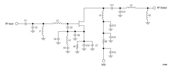
Figure 9. SKY65052-372LF Evaluation Board Schematic
