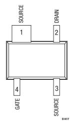
Figure 2. SKY65052-372LF Pinout – 4-Pin SC-70 (Top View)
