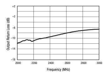
Figure 6. Output Return Loss vs Frequency Over Temperature (PiN = -20 dBm)
