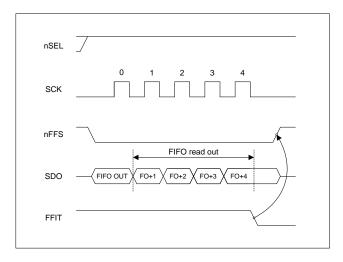
During FIFO access  $f_{SCK}$  cannot be higher than  $f_{ref}/4$ , where  $f_{ref}$  is the crystal oscillator frequency.
