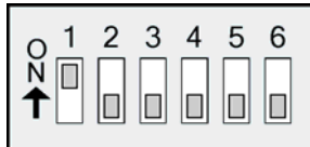
Figure B-08. RS-232 DIP Switch Settings
