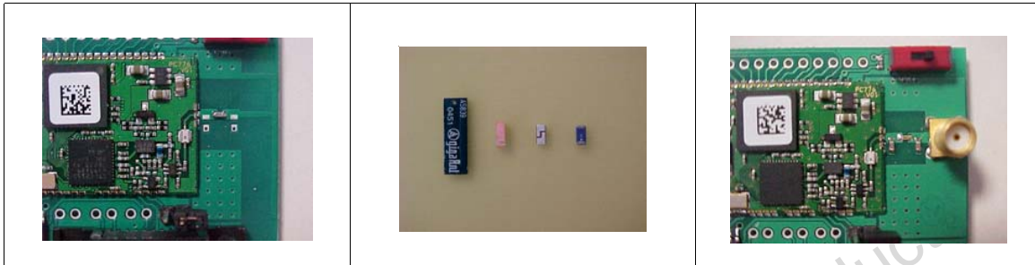
Figure 5. SMA connector for external antenna
