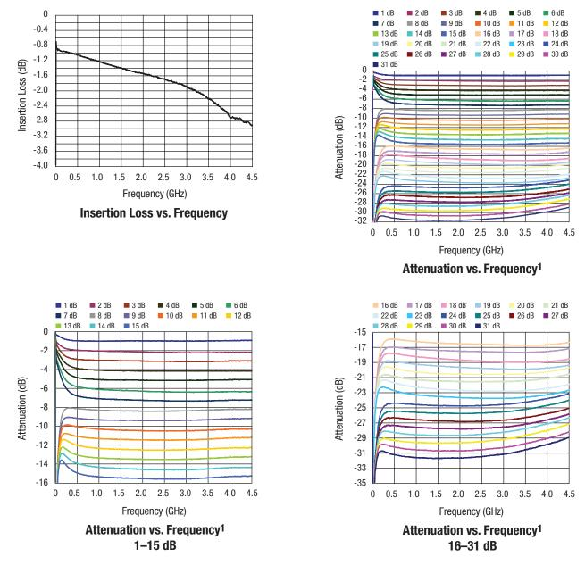
1. Attenuation normalized to insertion loss
