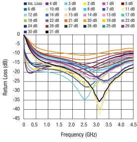
Input Return Loss vs. Frequency
