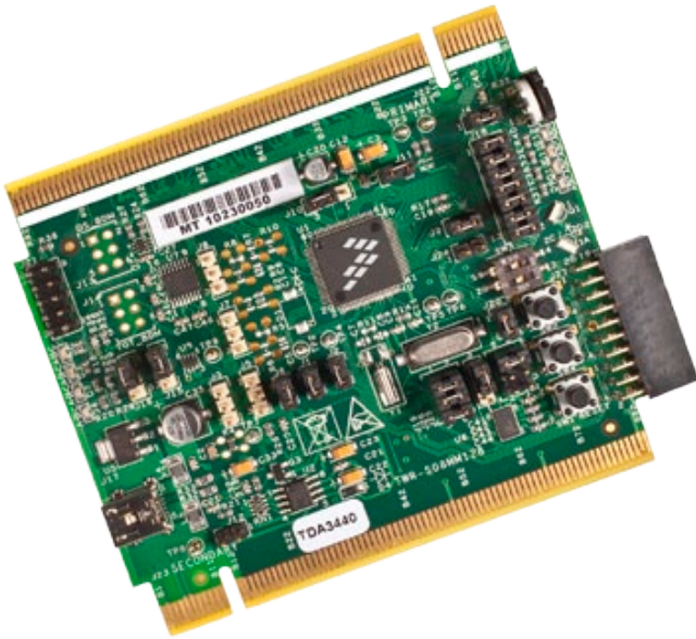
Figure 3: TWR-S08MM128 with Default Jumpers Used in Table 1
