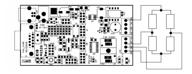
Pay attention to the connection of INP and INM, the differential signal INP-INM from the sensor has to be positive.
