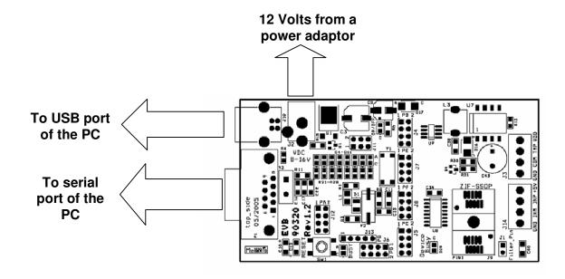
For the serial connection a non crossed cable has to be used (see picture bellow).
