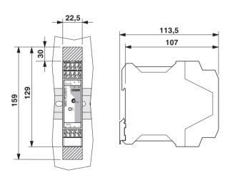
Mounting position: Installation depth 107 mm (+ DIN rail)
