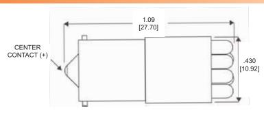
Measurements are typical Dimensions are inches [mm]
