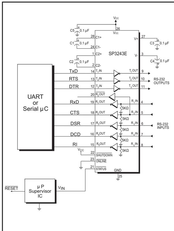
Figure 10. Interface Circuitry Controlled by Microprocessor Supervisory Circuit
