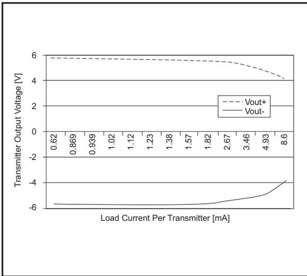
The SP3243E driver outputs are able to maintain voltage under loading of up to 2.5mA per driver, ensuring sufficient output for mouse-driving applications.
