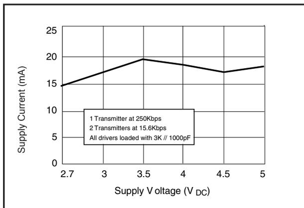
Figure 5. Supply Current VS. Supply Voltage for the SP3243EU
