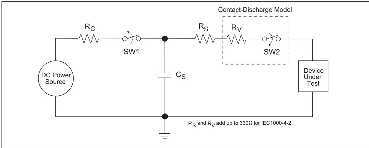
Figure 24. ESD Test Circuit for IEC1000-4-2
