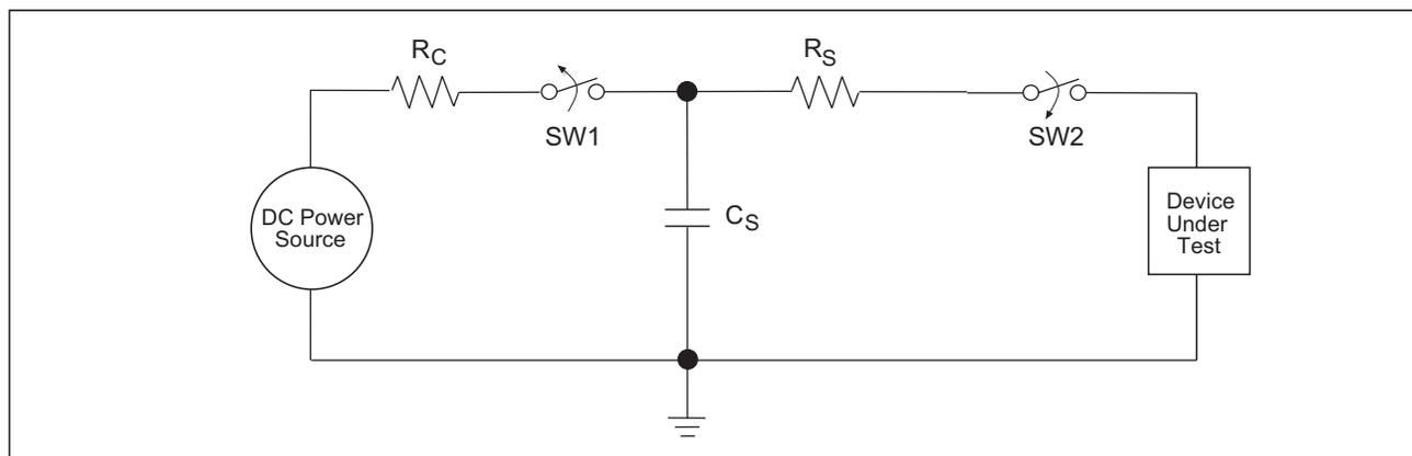
Figure 23. ESD Test Circuit for Human Body Model
