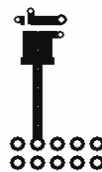
b. 125\text{ }^\circ\text{C}/\text{W} when mounted on a minimum pad of 2 oz copper
