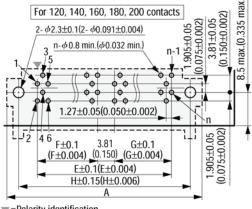
Recommended PCB Thickness  $t=1.6\pm0.19(0.063\pm0.007)$ "n" is number of contacts.
