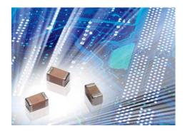
The QM series has been designed to significantly reduce noise characterstics while providing high capacitance values and a low voltage coefficient, making it ideal for mobile phone, hard disk drive, and LCD panel driver circuit application. QM series is based on X5R temperature characteristics with temperture variation of capacitance within +15% from -55°C to +85°C. This capacitance change is non-linear. Capacitance for X5R will also vary under applied voltage and frequency.
