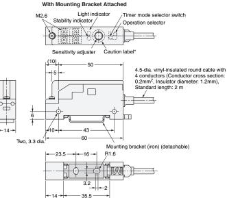
\*After adjusting the sensitivity, attach the caution label at the location indicated by  $\bigcirc$  above to prevent malfunction.
