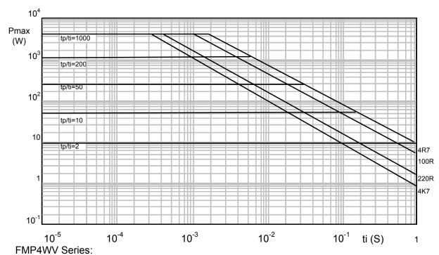
Pulse on a regular basis; maximum permissible peak pulse power (P-max) as a function of pulse duration  $(t_i)$ .
