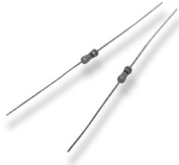
Metal glaze resistors are manufactured using thick film techniques. The ceramic slugs have the thick film applied, the film is fired and end caps are forced onto the slugs, the resistive element is spiralled to value and lead wires are welded onto the end caps. Four layers of coating are applied - the first being a phenolic resin, the other three being epoxy.
