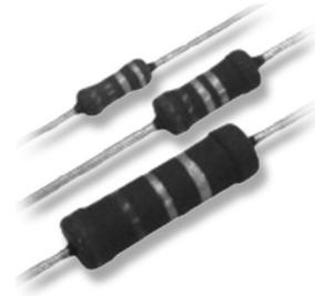
The RR Series is manufactured by depositing a homogeneous film of metal alloy onto a high-grade ceramic body. After a helical groove has been cut in the resistive layer, tinned connecting wires of electrolytic copper are welded to the end-caps. The resistors are coated with a red, non-flammable lacquer, which provides electrical, mechanical and climatic protection. The coating is resistant to all cleaning solvents in accordance with MIL-STD-202, method 215 and IEC 60068-2-45.
