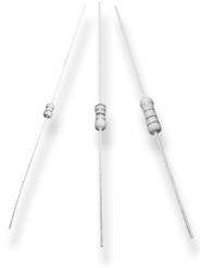
The resistive element comprises a thin film of carbon, deposited onto a high thermal conductivity ceramic core. Metal end caps are force fitted to the element prior to spiralling to value. Tinned copper lead wires are welded to the end caps and the components are then coated. One coat of phenolic resin is followed by three coats of epoxy resin. All resistors are tested for value and tolerance.
