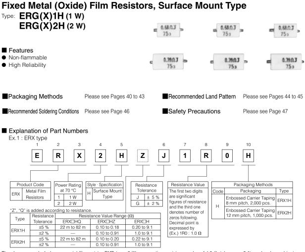
The above example 1 shows a metal film resistor SMD type, 2 W power rating, resistance value of 1.0 Ω, tolerance ±5 %, and embossed taping.
